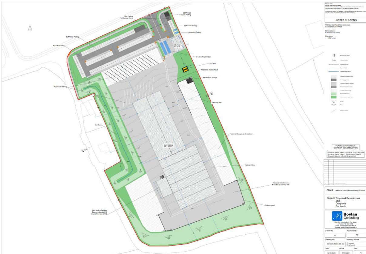
Figure 3-1 Indication of alternative broad layout considered at an early stage in the design process. This broad layout included the in-take / out-take area of the main building located to the north, and the processing and services area located to the south.
