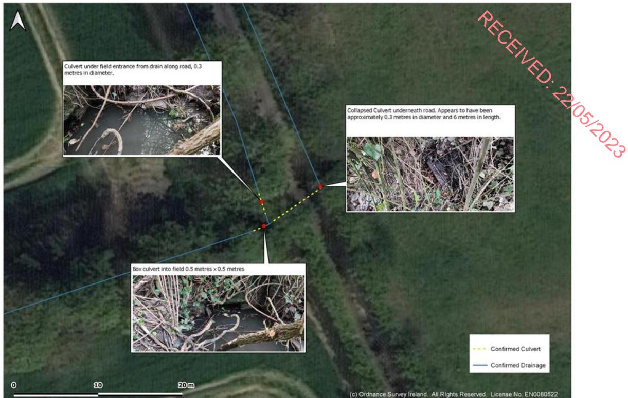
Figure 5-15 Drainage arrangement beneath local road south of site
