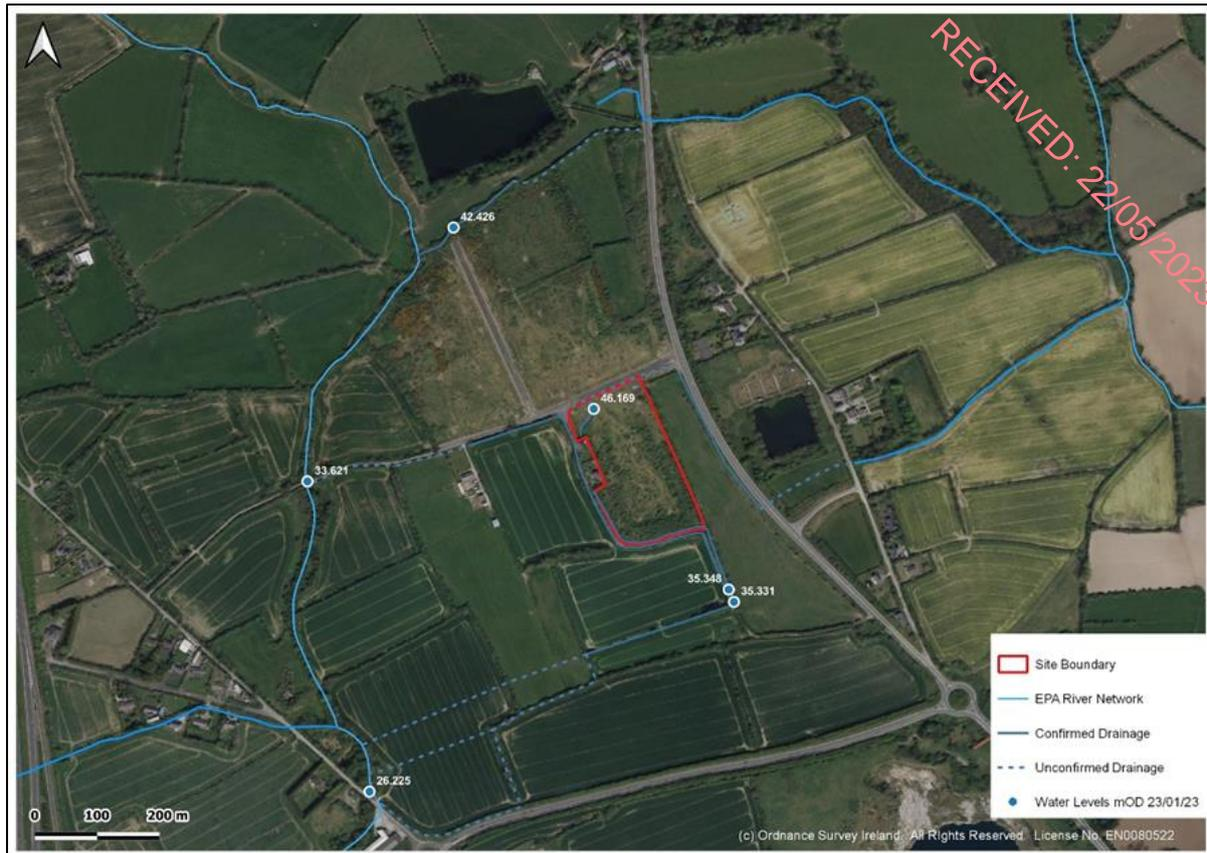
Figure 8-5 Drainage network downstream of site
