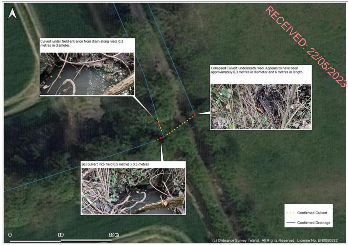
Figure 8-4 Drainage arrangement beneath local road south of site
