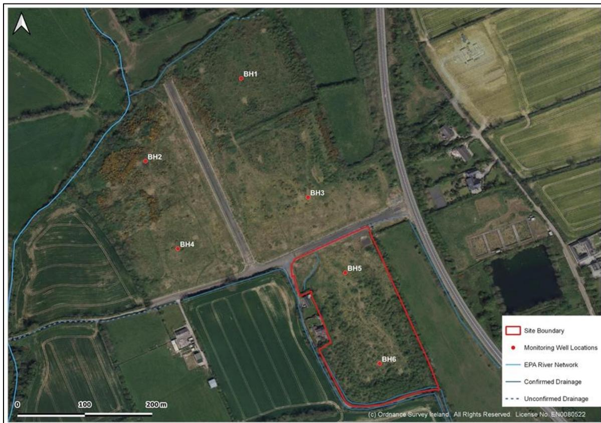
Figure 8-7– On-site groundwater monitoring wells
