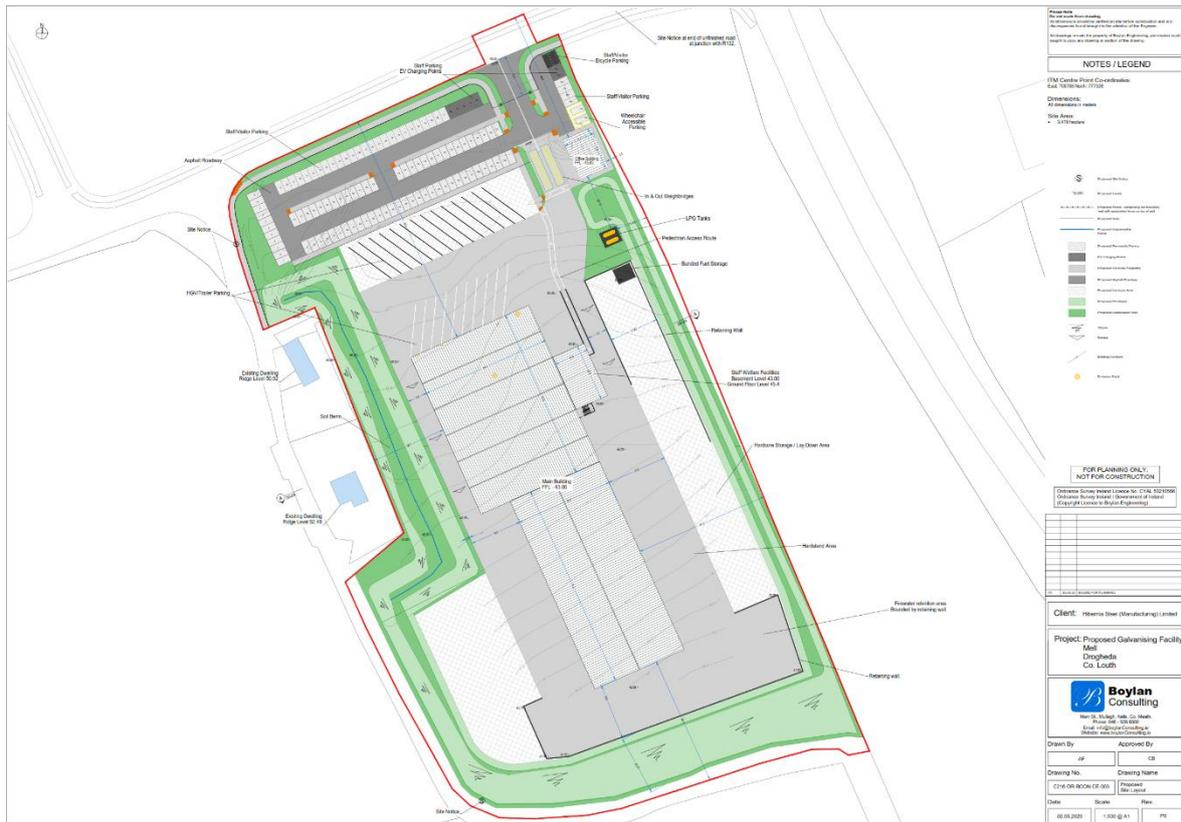
Figure 6-1 The proposed development galvanising plant layout.
